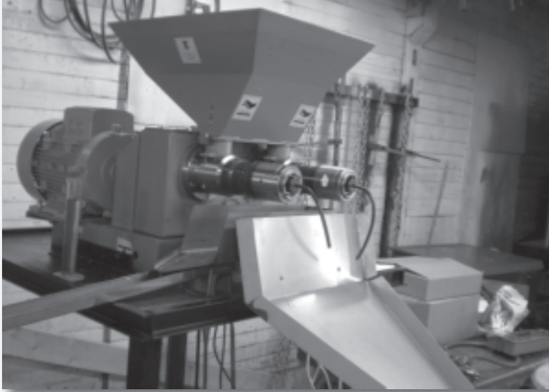
Is it possible to press out the fuel on the farm? Penn State University found this "portable," on-site press capable of producing enough SVO to run both pieces of equipment.
