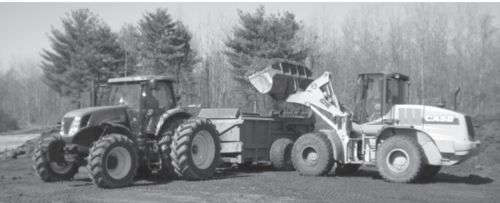
Elsbett systems were installed in a T7060 New Holland tractor and a Case 621E wheel loader, both with tier 3 engines and common rail, high pressure fuel systems, then the specially equipped units were transported to Penn State.
